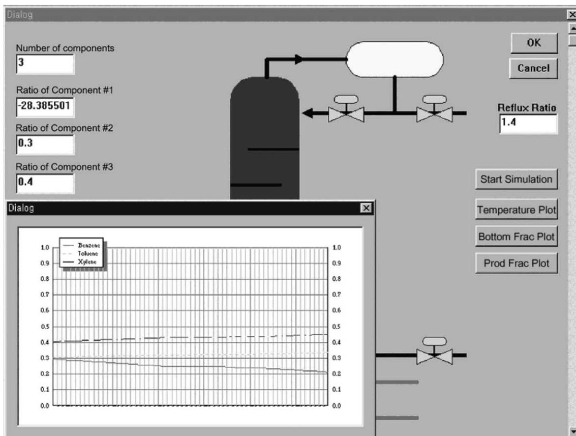
Fig. 4. Screenshot of a main client program of the second generation of the implementation.
