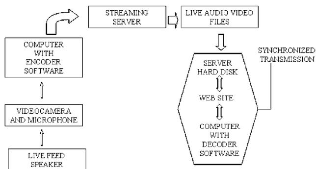
Fig. 1. Illustration of a simple videoconferencing system in a network.
